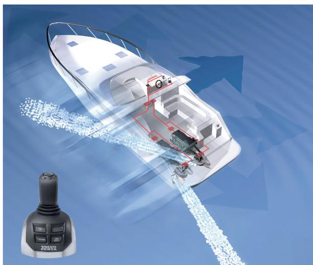
With the joystick the driver can now maneuver the boat, at low speed. The joystick is coupled to a sophisticated and specially developed software that individually commands the electronically controlled engines and underwater units of the system to steer, throttle and shift gears independently, making the boat move in any direction the driver wants – sideways, diagonally, forward, backward or rotate – with just one hand.
